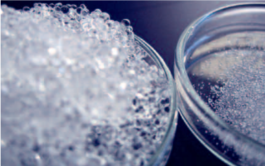
Picture of Flocare GB 300 before (right) and after (left) water absorption
