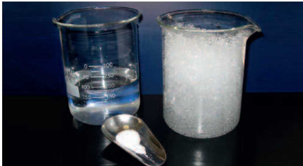
GB300 absorption: 1 g GB300 + 200 mL water = 500 mL swelled beads
